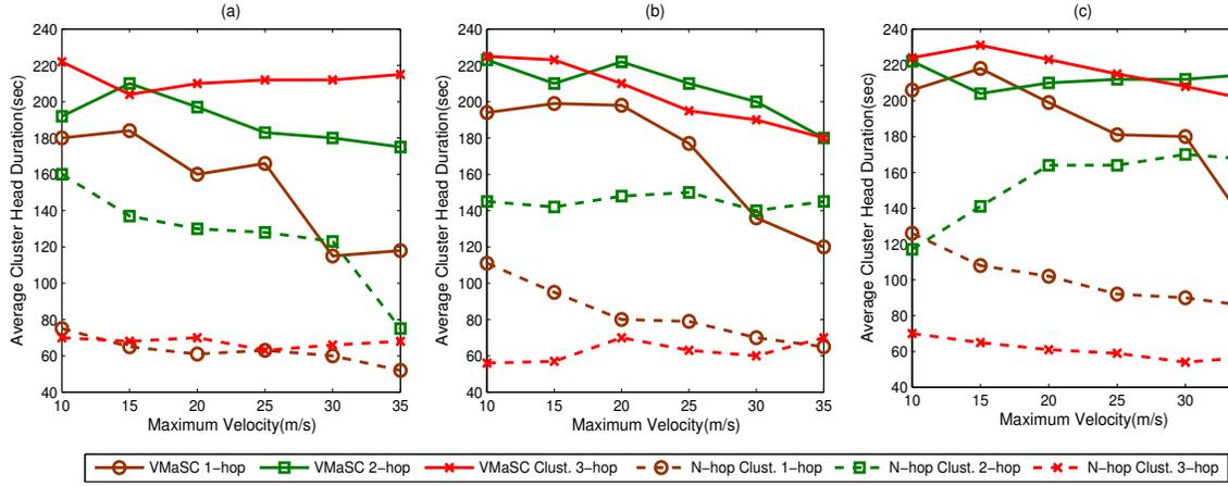
Fig. 2. Average cluster head duration, for transmission range (a) 100m (b) 200m (c) 300m
