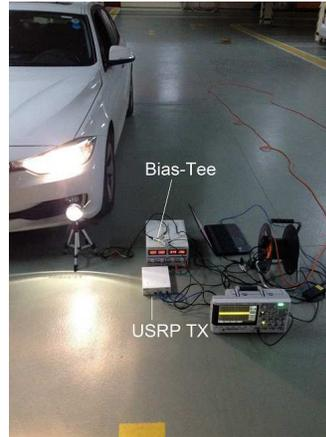
Figure 3: Transmitter Unit
