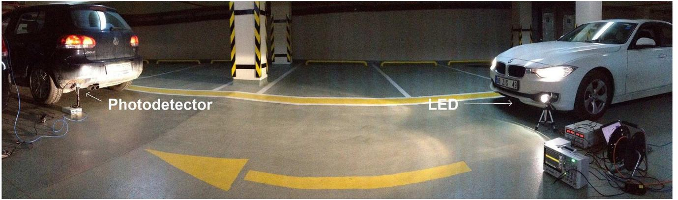
Figure 1: Vehicular VLC experimental setup.
