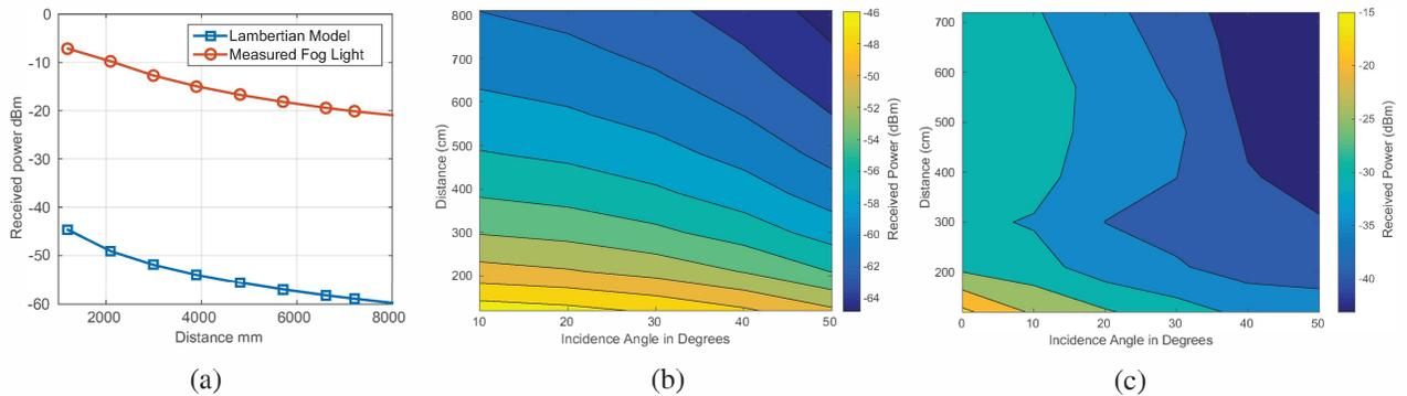
Fig. 3: (a) Lambertian vs. Off-The-Shelf Fog Light (b) Estimated Lambertian Pattern (c) Single Channel Fog Light Pattern
