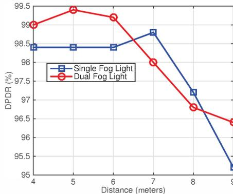
Fig. 6: DPDR performance of single and dual channel VLC
