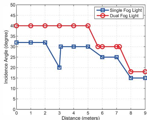
Fig. 5: Single and Dual LED Fog Light Usage Limits
