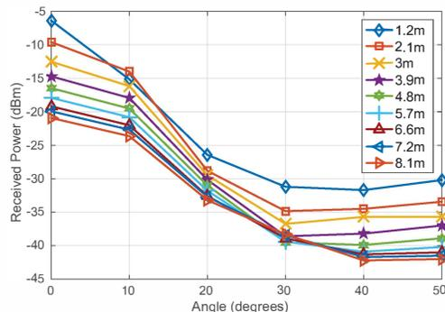
Fig. 4: Received Power With Varying Angle and Distances
