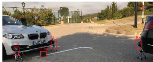
Fig. 1: Vehicular VLC Experimental Setup
