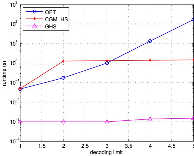
Fig. 2. Average runtime for different decoding limits in a 20-link network.
