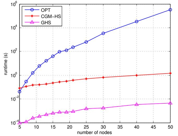
Fig. 4. Average runtime with the decoding limit  $K = 5$  for different number of nodes.
