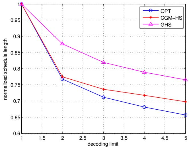
Fig. 1. Normalized schedule length for different decoding limits in a 20-link network.
