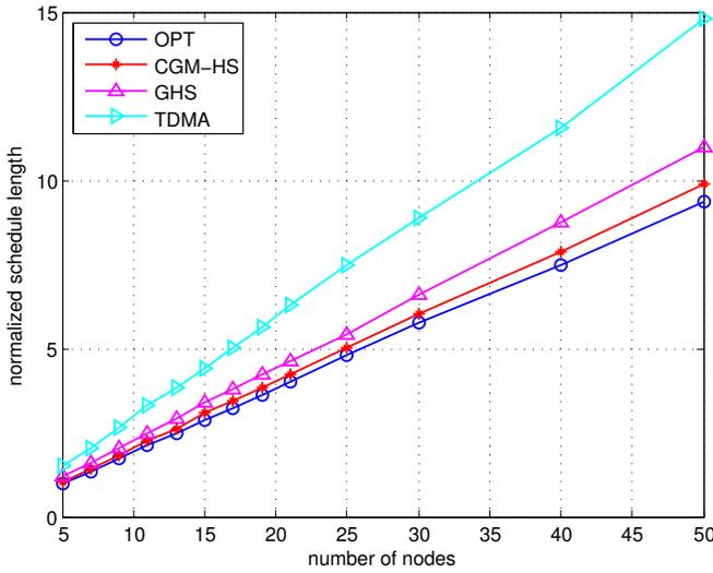
Fig. 3. Normalized schedule length with the decoding limit  $K = 5$  for different number of nodes.
