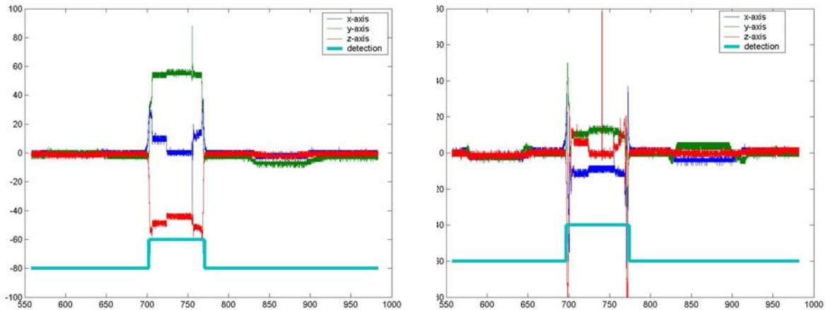
**Figure 3** Raw samples of  $mag(x)$ ,  $mag(y)$ ,  $mag(z)$  and detection flag of the sensor node in the middle (left) and end (right) of the parking space; time (x-axis) is in seconds
