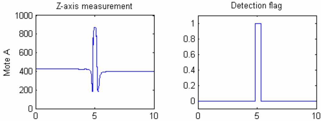
**Figure 2** Raw samples of  $mag(z)$  and detection flag of a sensor node near an intersection; time (x-axis) is in seconds
