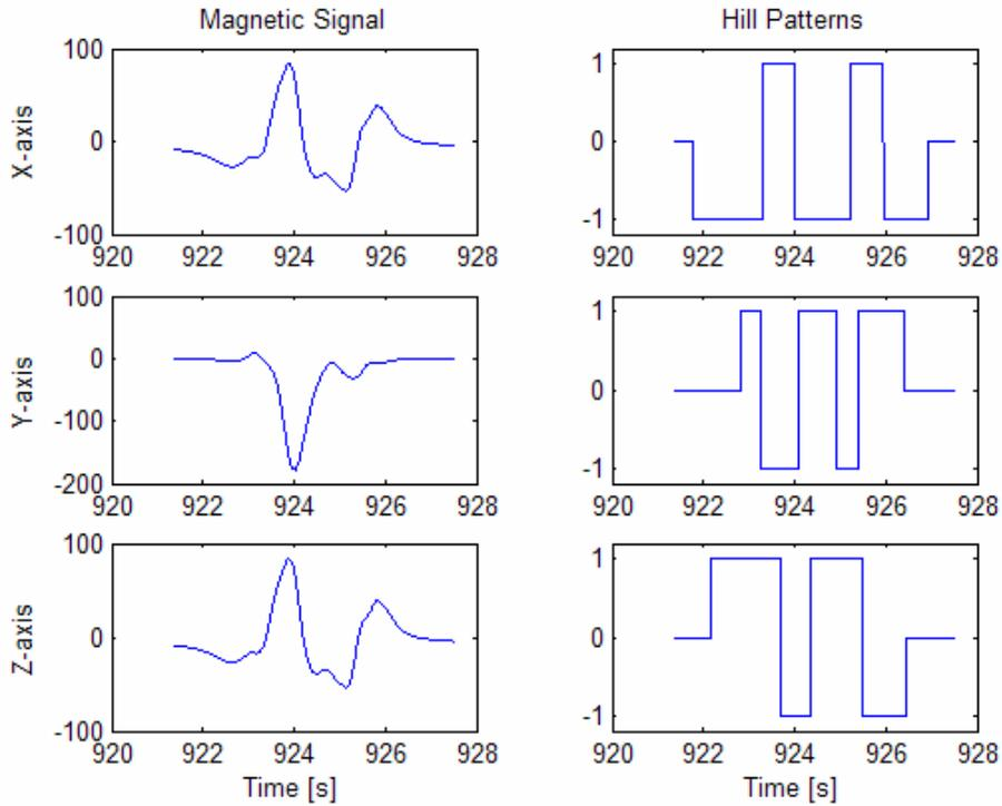
Figure 7 Magnetic signals and hill patterns from two trucks of FWHA class 5
