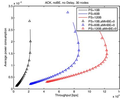
Fig. 6. Power consumption versus net throughput for different  $BE$  parameter settings.
