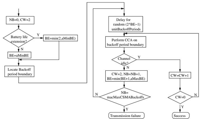
Fig. 1. Backoff mechanism for 802.15.4 CSMA
