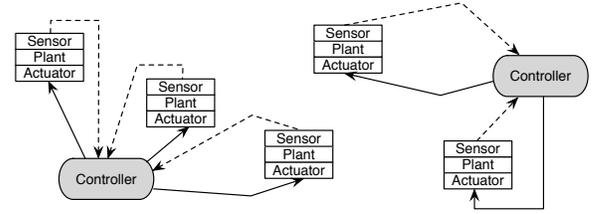
Fig. 1. Overview of the WNCS setup.
