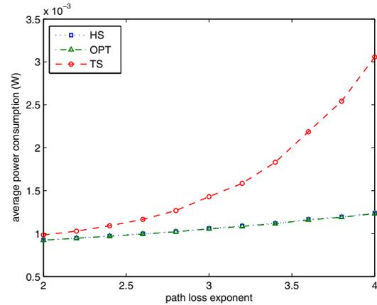
Fig. 7. Average power consumption for different path loss exponent values in a network of 20 nodes where nodes are uniformly distributed within a circular area of radius 5 m,  $\Delta = 10$  ms and  $\Omega = 100$  ms.
