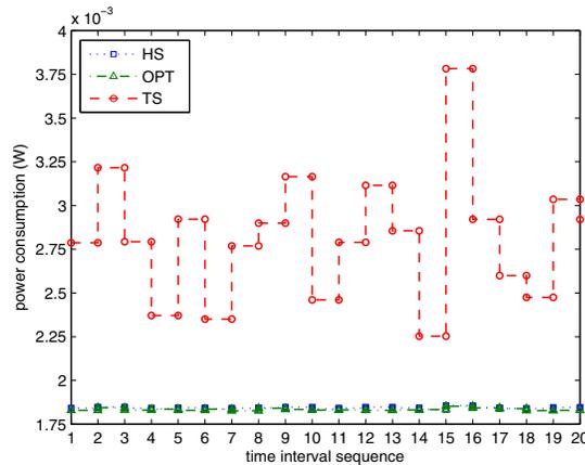
Fig. 9. Power consumption in a network of 20 nodes under Nakagami fading with  $m = 3$  where nodes are uniformly distributed within a circular area of radius 5 m,  $\Delta = 10$  ms and  $\Omega = 100$  ms.
